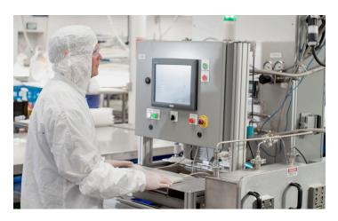
Standard Labtainer Pro BPCs are inspected after manufacturing, prior to being packaged and shipped. We also conduct a 100% helium integrity test, helping to ensure that our product has the highest standards of quality when it's delivered to the customer.
